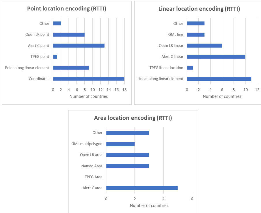
Figure 19: Location referencing methods used for the exchange of RTTI-related information
